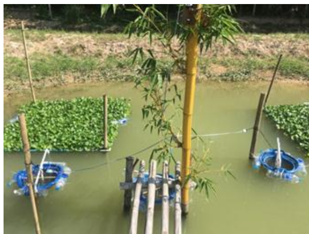
Figure 2. The volcanic rock bioreactors and quadrats filled with water hyacinth were placed into each aquaculture pond.
